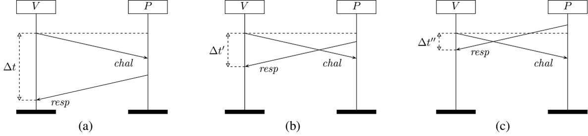
Figure 1: Three timing scenarios of a challenge/response round.
